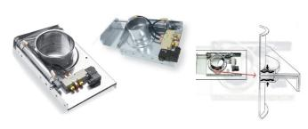
Truly "air-tight" blast gates operate manually or pneumatically and utilize a two part, self-sealing gasket assembly to completely isolate outside air, guaranteeing no air leakage across the valve or into the atmosphere. Designed to withstand 16 Hg" of negative pressure. Available in Zinc Plate or Stainless Steel.
