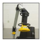
The Dust Extraction Swing Arm safely removes airborne dusts, gases and smoke emitted during the manufacturing process.
